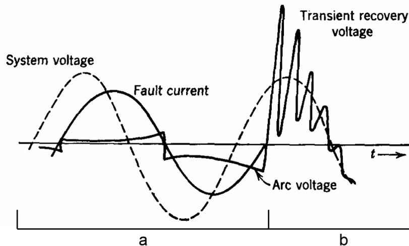
Figure 6: Typical oscillatory transient resulting from clearing of network faults [6].
