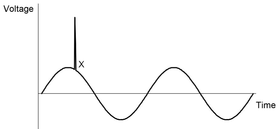
Figure 1: A typical impulsive transient shown at point X.
