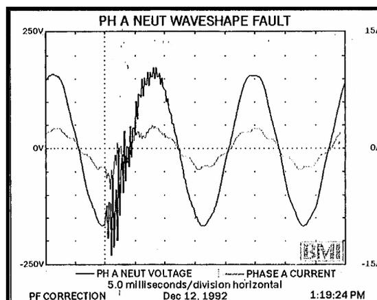
Figure 4: Voltage and current transients resulting from capacitor bank energisation [5].
