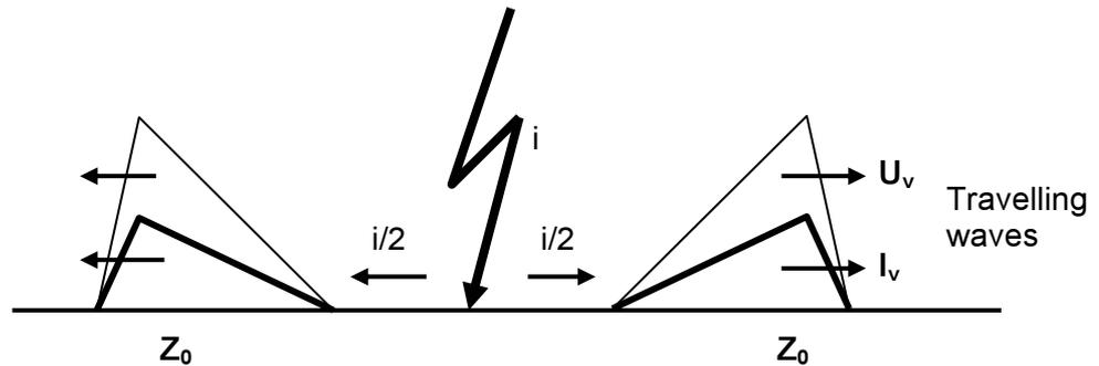
Figure 7: Travelling waves due to a lightning strike.
