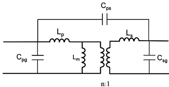
$C_{pg}$  is the effective capacitance of the primary winding to earth.
