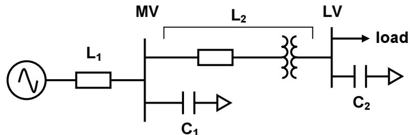
Figure 5: Power system network conducive to magnification of capacitor switching transients
